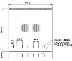
TOP VIEW - 600 DEEP WR CABINET WITH REAR HINGE BOX SECTION
